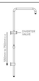
Mark down vertical between 550mm and 750mm from centre of water outlet. Warning: Ensure no water pipe or power cable in wall at this location.
