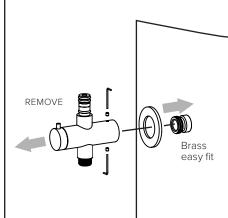
Loosen grub screws on body of diverter valve using a 2.5mm allen key. Withdraw the brass easy fit. Screw easy fit onto water outlet till it is flush against the wall face; slide chrome
