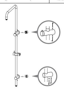
Fit the entire assembly onto wall by tightening the grub screws on the bottom and top mounting bracket using the 2.5mm allen key.
