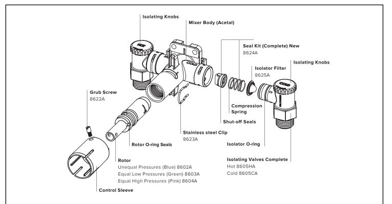
A rubber shut-off seal and spring is fitted in each of the two inlets of the valve body and two O-ring seals fitted to the rotor located inside the valve body.
