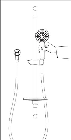
6. Screw the elbow into the water outlet (wingback). Sealant required on thread to achieve a water tight seal.
