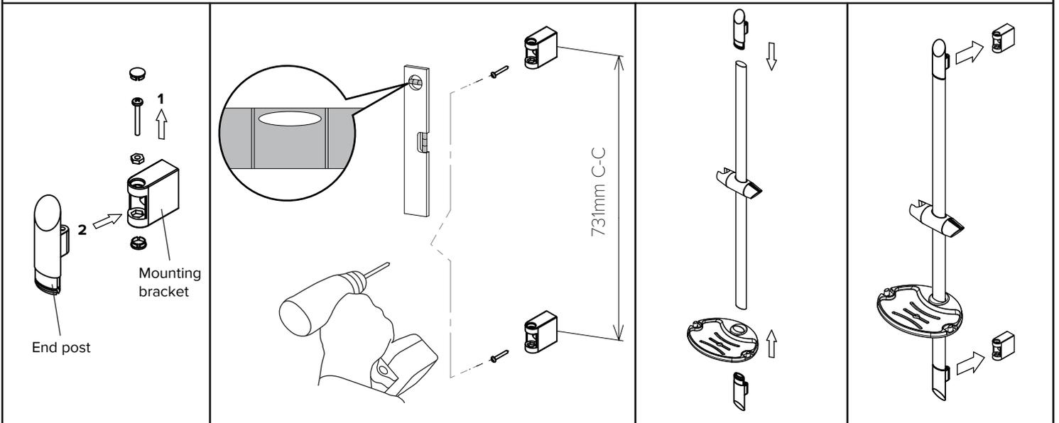
1. Unscrew and separate the mounting bracket from the end post.
