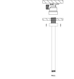
2. Apply seal thread tape to BSP and thread the vertical arm into the wingback.
