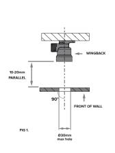
Ensure the wingback when fitted is parallel and square to the finished ceiling lining as shown (fig 1).
